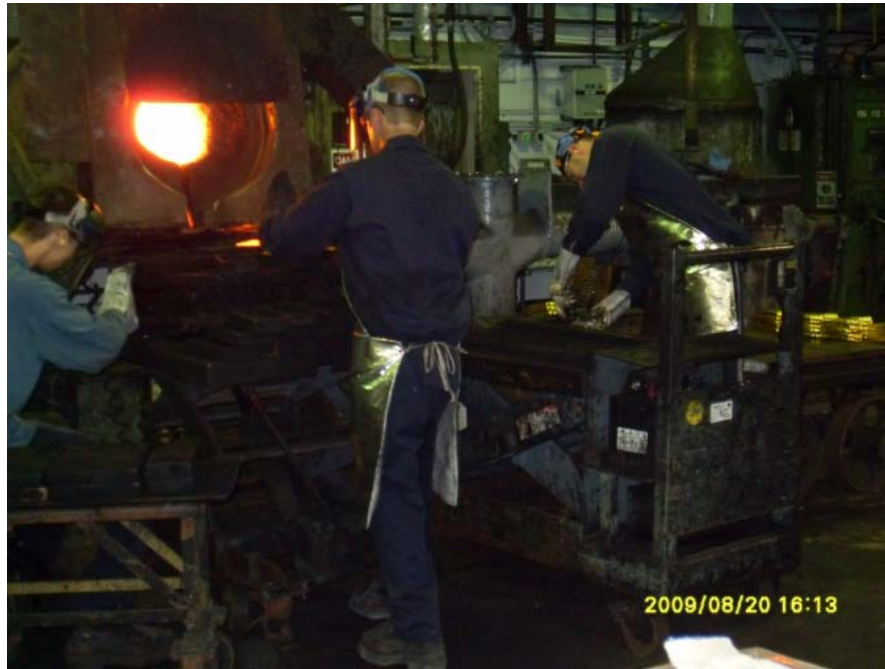
Photo 3 – Pouring, Quenching & Stacking 995 Anodes
