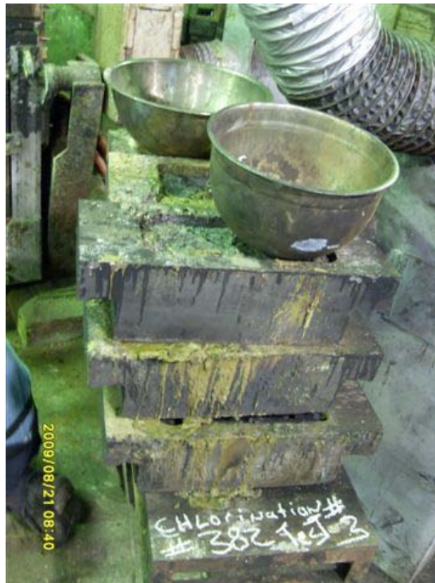
Photo 4 –Moulds of Slag taken from Chlorination Batch 90382 ready to be demoulded and remelted
