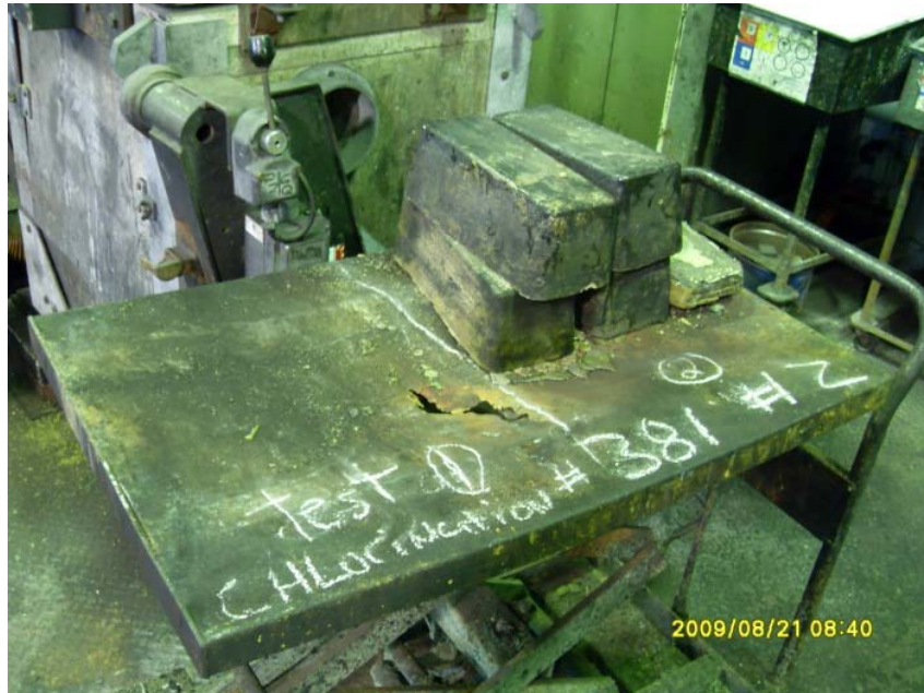
Photo 5 – Demoulded Slag from Chlorination Batch 90381 ready to be remelted
