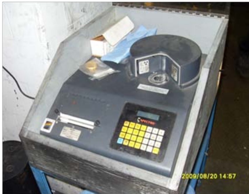
Photo 2 – XRF Machine used to analyze dip samples from the chlorination furnace to determine if gold is refined to 995 or better
