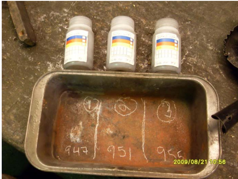
Photo 7 – Timed Slag Dip samples bottled for transport to Assay Lab
