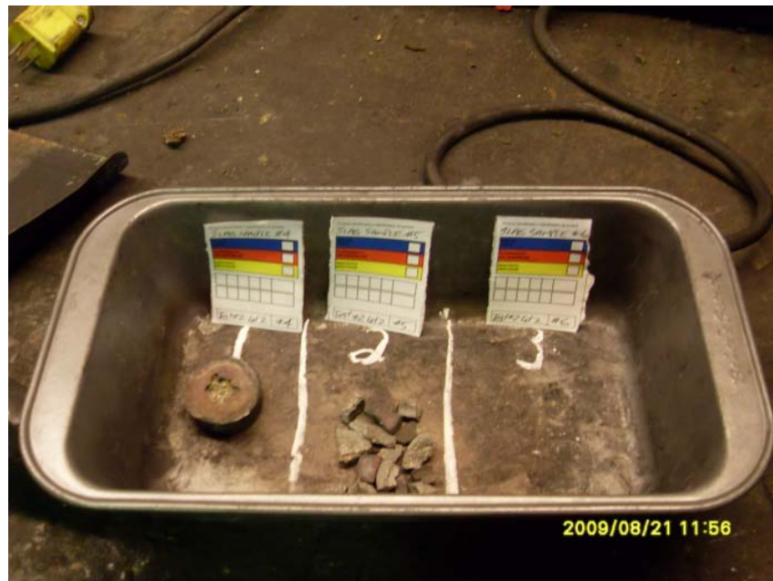
Photo 6 – Timed Slag Dip samples drawn from remelted Slag
